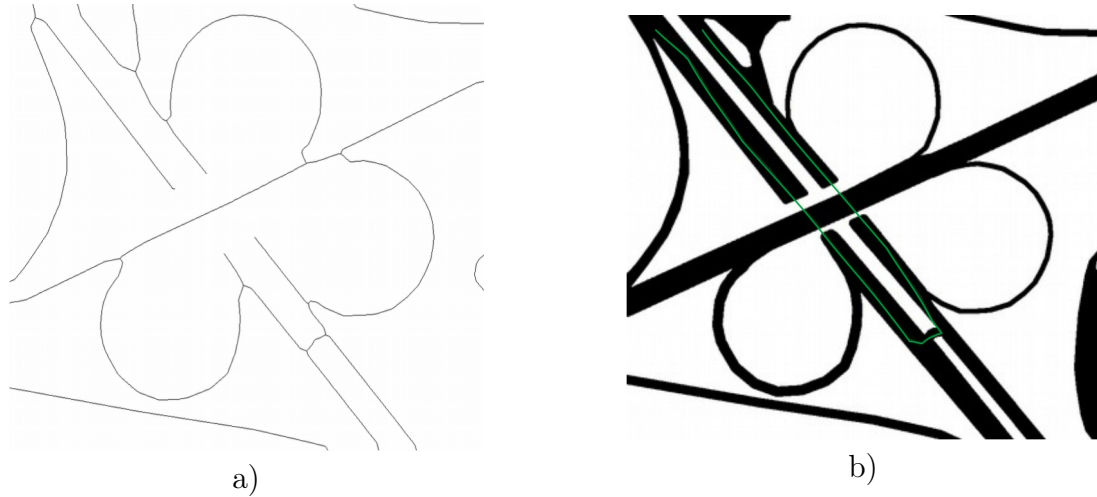
Fig. 4. a) skeleton based on a binary image; b) SRN binary image with green color indicating path for GPX track
